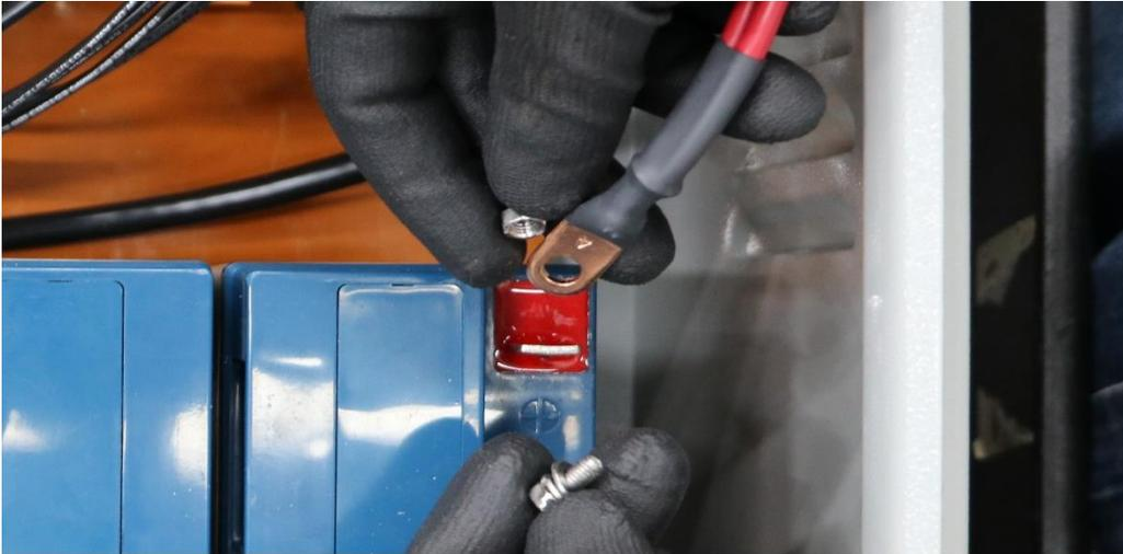
Figure 9: Remove Power and Ground Cable
