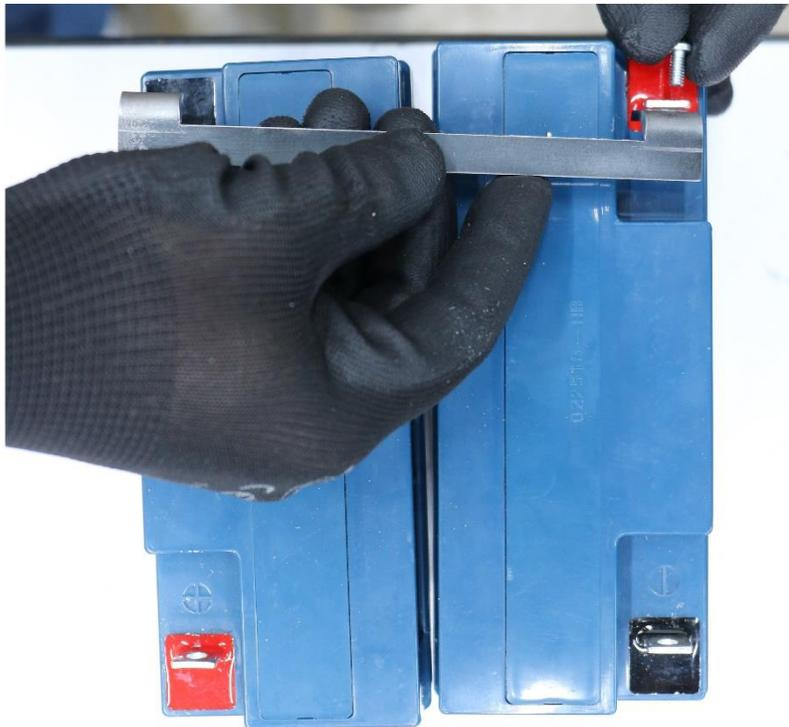
Figure 12: Bus Bar Holding Two Batteries
